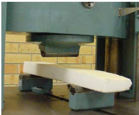
(a) Laminated un-reinforced PU foam
